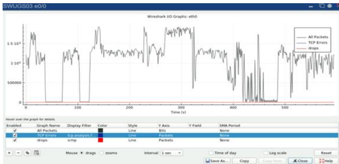
Fig. 10 -Excessive traffic on the circuit between SWUGS_03 and SWUGS_01. Source: Own authorship.
