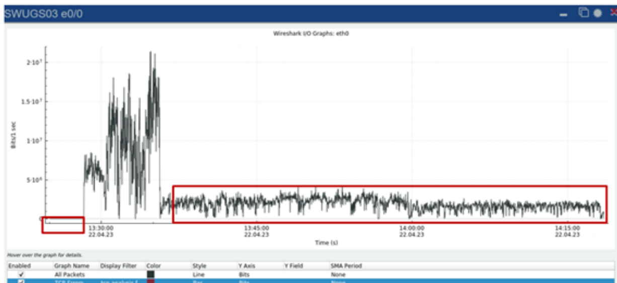
Fig. 20 - Automatic traffic balancing in SWUGS. Source: Own authorship.
