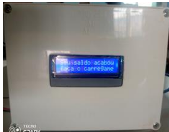
Fig. 16 -Final meter interface indicating no recharge. Source: (Author's own, 2024).
